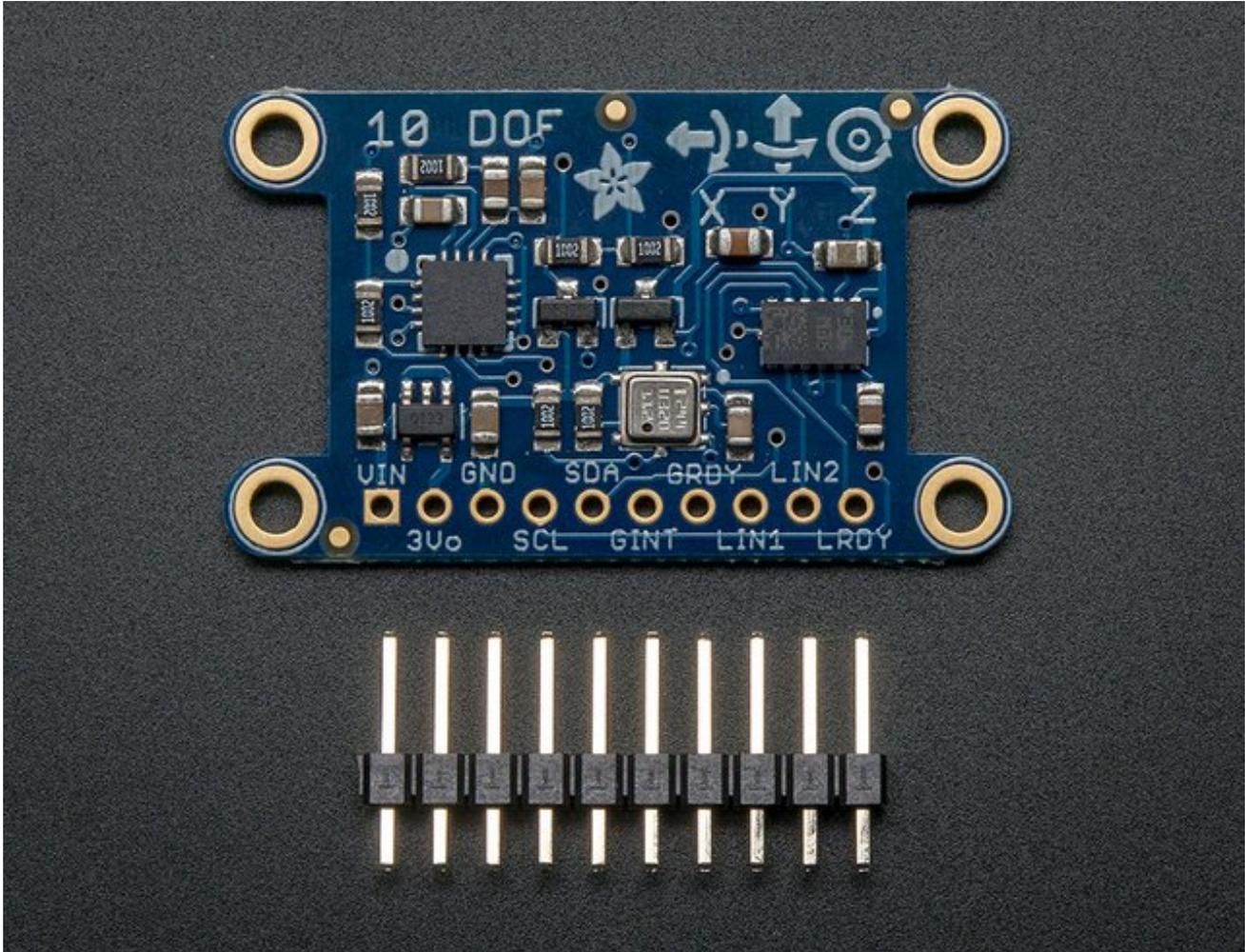
Please note that there is a small cosmetic error on the first revision of these boards (shown above). The straight X arrow for the accelerometer should be pointing in the opposite direction, towards the right. This will be fixed in the net run of these boards. Adafruit's 10DOF (10 Degrees of Freedom) breakout board allows you to capture ten (err, eleven!) distinct types of motion or orientation related data.
