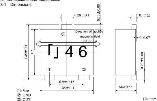
Coplanarity: less than 0.1mm(includiong under reflow condition)
