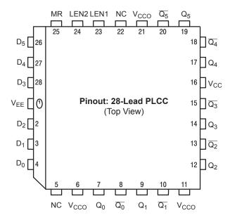
$<sup>^{\</sup>star}$  All  $V_{CC}$  and  $V_{CCO}$  pins are tied together on the die.
