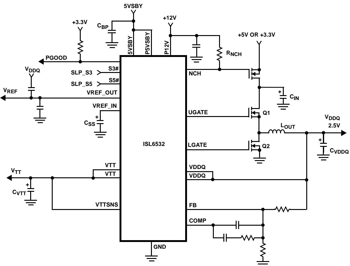
**Typical Application - Input From 5V Dual**
