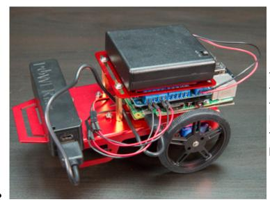
Finish the robot by screwing the top plate firmly to the standoffs in the center. Use double sided foam tape or electrical tape to hold the 4xAA battery pack to the top plate, and the USB battery pack to the front of the robot.
