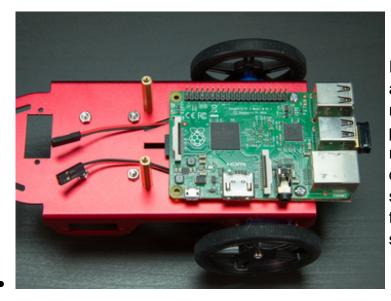
Place the Pi on the cardboard and position it so the Pi's rear mounting holes (near the USB ports) are directly above the long mounting slot at the back of the chassis. Use the #4-40 machine screws and nuts to screw through the Pi and cardboard to securely hold the Pi in place.
