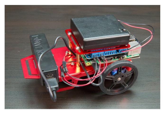
This is a fun project to build a simple robot using the Raspberry Pi and Adafruit's awesome robot chassis kit (http://adafru.it/2939). This robot is one of the simplest robots you can build and uses two DC motors to control a pair of wheels. A swivel caster in the front holds the robot up, and the Raspberry Pi with motor HAT (http://adafru.it/2348) controls the motors.
