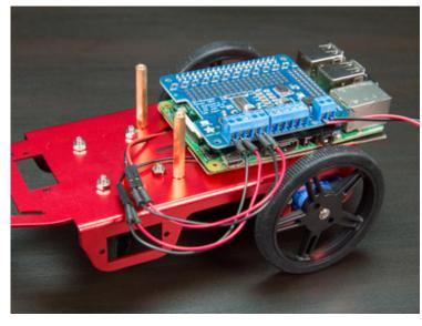
right (or 'passenger side') DC motor should be connected to port M2 on the motor HAT.
