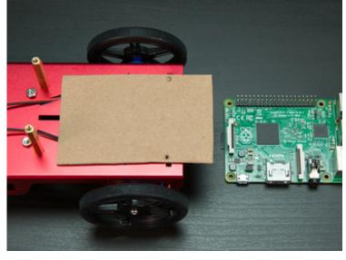
size as the Raspberry Pi. This cardboard will protect the bottom of the Pi from touching the metal robot chassis and shorting out. It's very important to prevent the bottom of the Pi from touching the metal chassis or you could damage the Pi!
