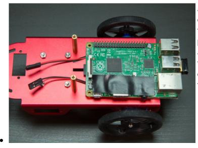
across the HDMI connector side of the Pi. This will help prevent the motor HAT from getting pushed down into the connectors and shorting out. If you are using the standoffs you can place them over the front mounting holes of the Pi (not shown).
