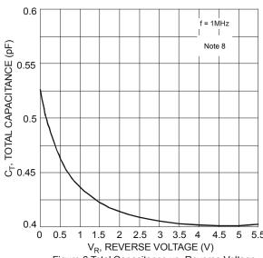
Figure 6 Total Capacitance vs. Reverse Voltage
