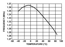
FIGURE 6. SWITCHING FREQUENCY vs TEMPERATURE
