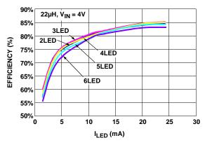
FIGURE 11. EFFICIENCY CURVE WITH 2, 3, 4, 5 AND 6 LEDs LOAD
