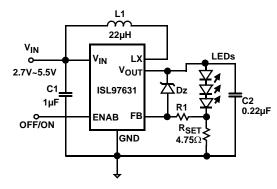
FIGURE 10. LED DRIVER WITH OVERVOLTAGE PROTECTION CIRCUIT
