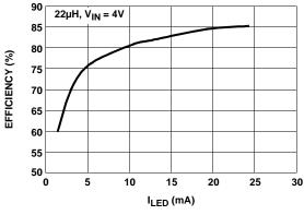
FIGURE 2. EFFICIENCY vs LED CURRENT (VIN = 4V)
