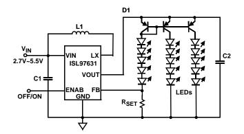
FIGURE 12. LEDs IN SERIES/PARALLEL WITH MIRROR CURRENT BALANCE
