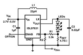
FIGURE 9. ANALOG DIMMING CONTROL APPLICATION CIRCUIT
